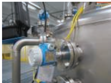
FIGURE 4. Vibronic point-level switches (left) are an active technology with constant self-check function built-in (right) to ensure functional integrity
